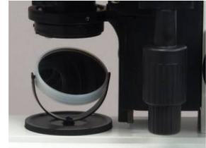
**Note:** The mirror is only used when there is a power failure or you are in the field and no power is available.
