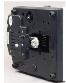
**Caution:** Before you turn over the microscope, be sure to take the eyepieces off and be certain that the head is securely locked by the thumb screw.
