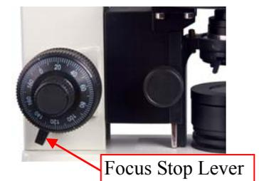
3.5.2 Turn the coarse focus knob until the specimen is in focus. Then use the fine focus knob to obtain a sharp image. You may now switch to another magnification objective.
