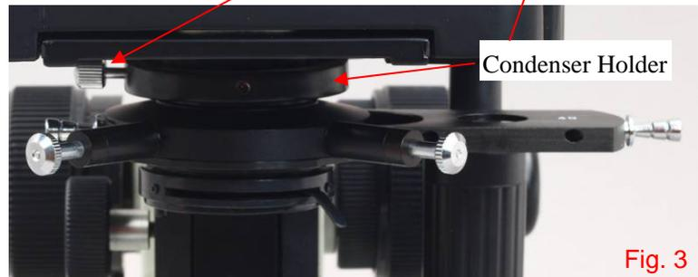
**Note:** there are 2 phase contrast objectives: 10X and 40X, and there are 2 condenser annular rings on the annular ring switch (3): 10X and 40X. The
